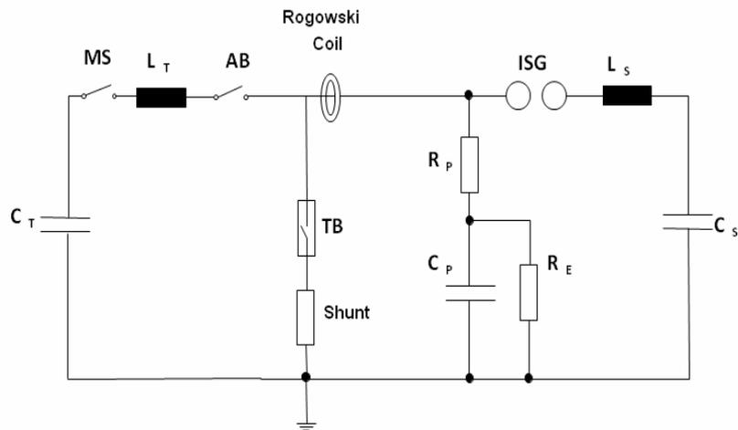
Fig. 2. Equivalent circuit diagram of a synthetic test circuit after Weil and Dobke used for the experimental testing
