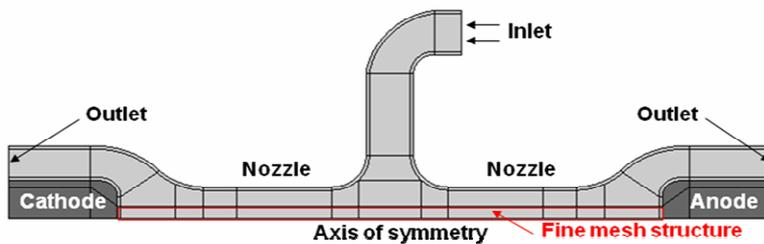
Fig. 3. Geometry for the CFD-simulations
