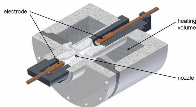
Fig. 1. Cross-sectional view of the circuit breaker model used in the experiments
