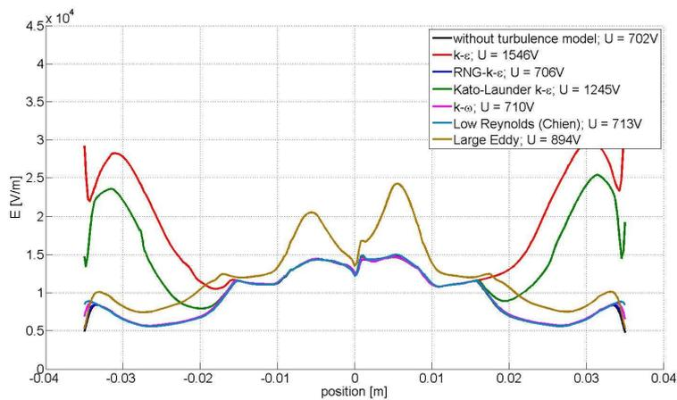
Fig. 6. Electric field along the axis of symmetry for simulations using different turbulence models at  $t=-1\mu s$
