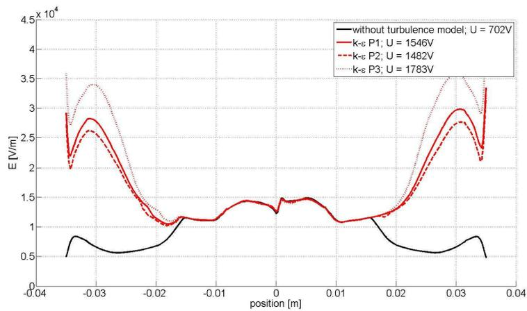
Fig. 5. Electric field along the axis of symmetry for simulations without turbulence model and simulations using the k-ε-turbulence model with different parameters at  $t=-1\mu s$
