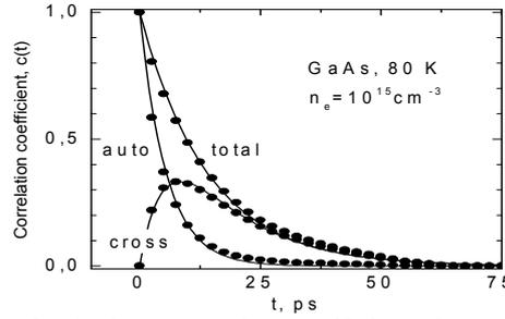
Fig. 3. Relaxation of velocity correlation coefficients in n-GaAs. Points - MC, curves - by equations (10).
