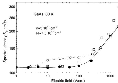
Fig. 2. Dependence of the spectral density of electron drift velocity fluctuations for compensated n-GaAs. MC with phonon, impurity and e-e scattering: (closed circles), without e-e scattering (diamonds). Experimental data—open squares [7].
