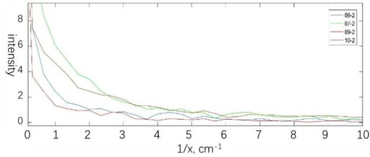
Figure 8. Fourier spectrum obtained by scanning in the direction of the flow (a) and in the direction perpendicular to the flow (b).
