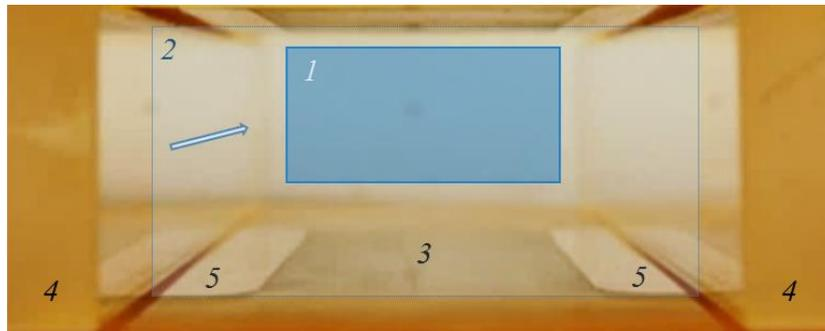
Figure: 2. Flow diagram in the shock tube: 1 – shock wave front, 2 - contact surface, 3 - surface discharge region, 4 - glasses, 5 - discharge electrodes. The arrow shows the direction of flow.
