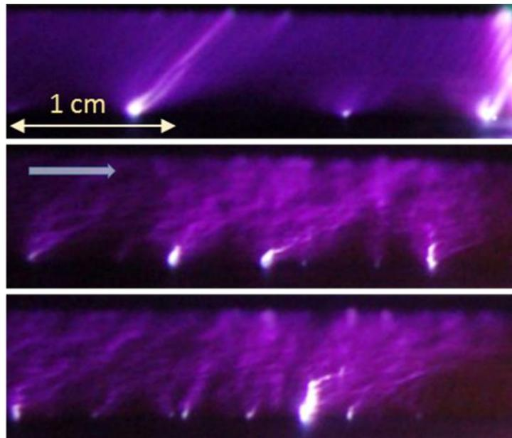
Figure: 4. Photographs of the discharge glow in a discharge chamber in still air (a), in supersonic airflows in turbulent boundary layer (b, c). The arrow shows the direction of flow.  $M_{\text{flow}}=1,52$ ,  $\rho_2=0.11 \text{ kg/m}^3$ .
