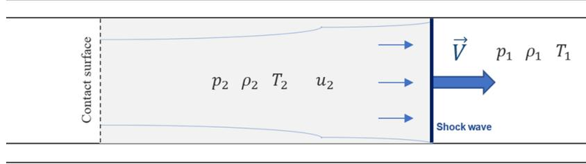
Figure: 3. The co-current flow behind the shock wave in the shock tube channel.
