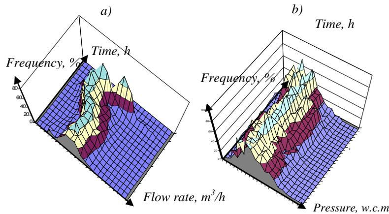
Fig. 2. Daily change in the frequency distribution of hydraulic operating parameters
