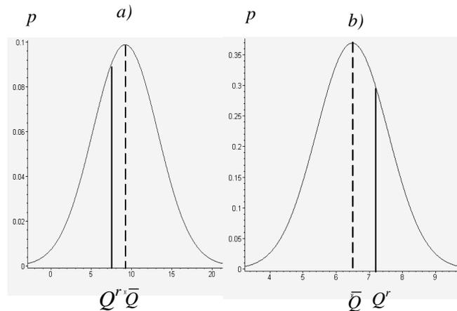
Figure 5. Illustration to the calculation of probability of providing consumer with a required flow rate: a) at node 2, b) at node 3.
