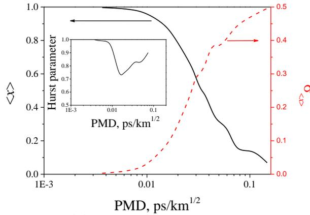
Fig. 2. Dependencies of  $\langle x \rangle$  (black solid curve), its standard deviation  $\sigma_{\langle x \rangle}$  (red dashed curve), and the corresponding Hurst parameter (inset) on the PMD parameter for  $\vec{p}=(1,0,0)$  and  $\vec{s}=(1,0,0)$ .
