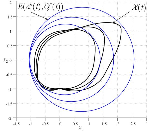
**Fig. 1.** Reachable sets  $\mathcal{X}(t)$  and their external estimates  $E(a^*(t), Q^*(t))$  for  $t = 0.14; 0.26; 0.4$ .
