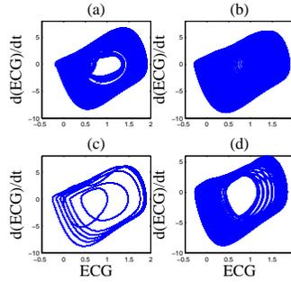
**Fig. 5.** Phase space of ECG without applying the control process. (a)  $k_{SA-AV} = 6.42$ , (b)  $k_{SA-AV} = 7.57$ , (c)  $k_{SA-AV} = 7.64$ , (d)  $k_{SA-AV} = 10$ . (a), (b) and (d) demonstrate non-periodic and unstable responses, and (c) represents periodic and stable response.
