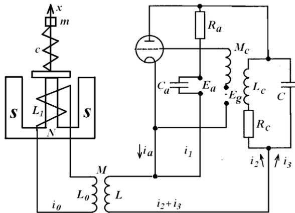
Fig. 1. Schema of a shaker with an amplifier interacting with an oscillator .
