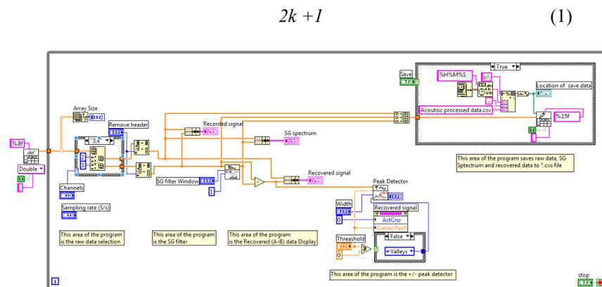
Figure 1: Block diagram of LabVIEW de-convolution software
