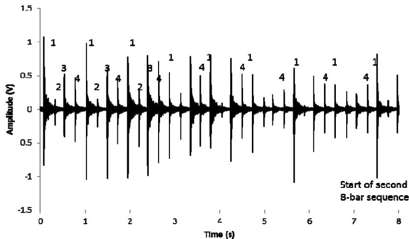
Figure 3: Decoding of the recovered male percussive impact sequence.
