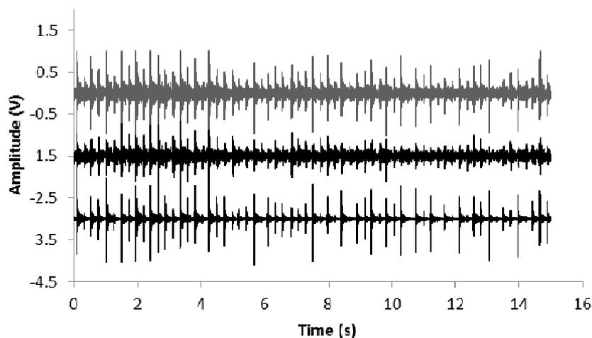
Figure 2: Bare foot recording and its de-convolution. Upper trace is the raw recording, middle the synthetic floor and lower trace depicts the step sequence.
