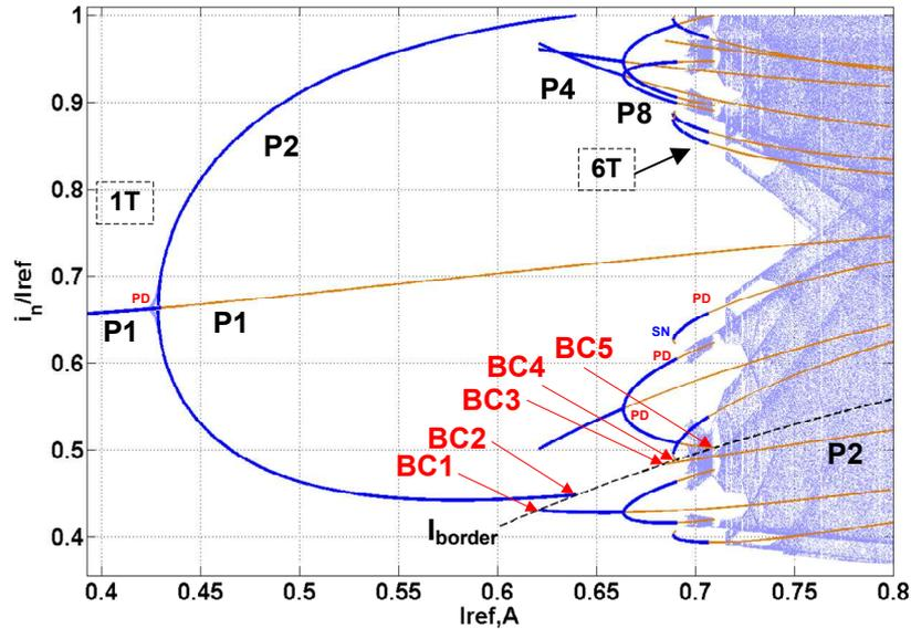
Fig. 4. The complete bifurcation diagram for  $S_c=200$  (A/s).
