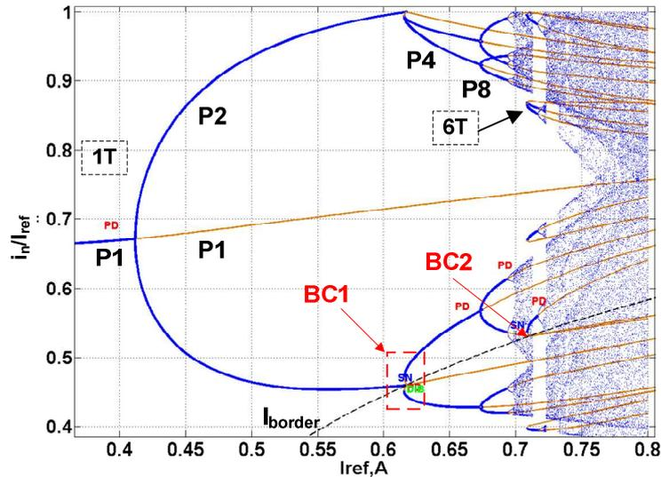
Fig. 3. The complete bifurcation diagram for  $S_c=0$  (A/s).
